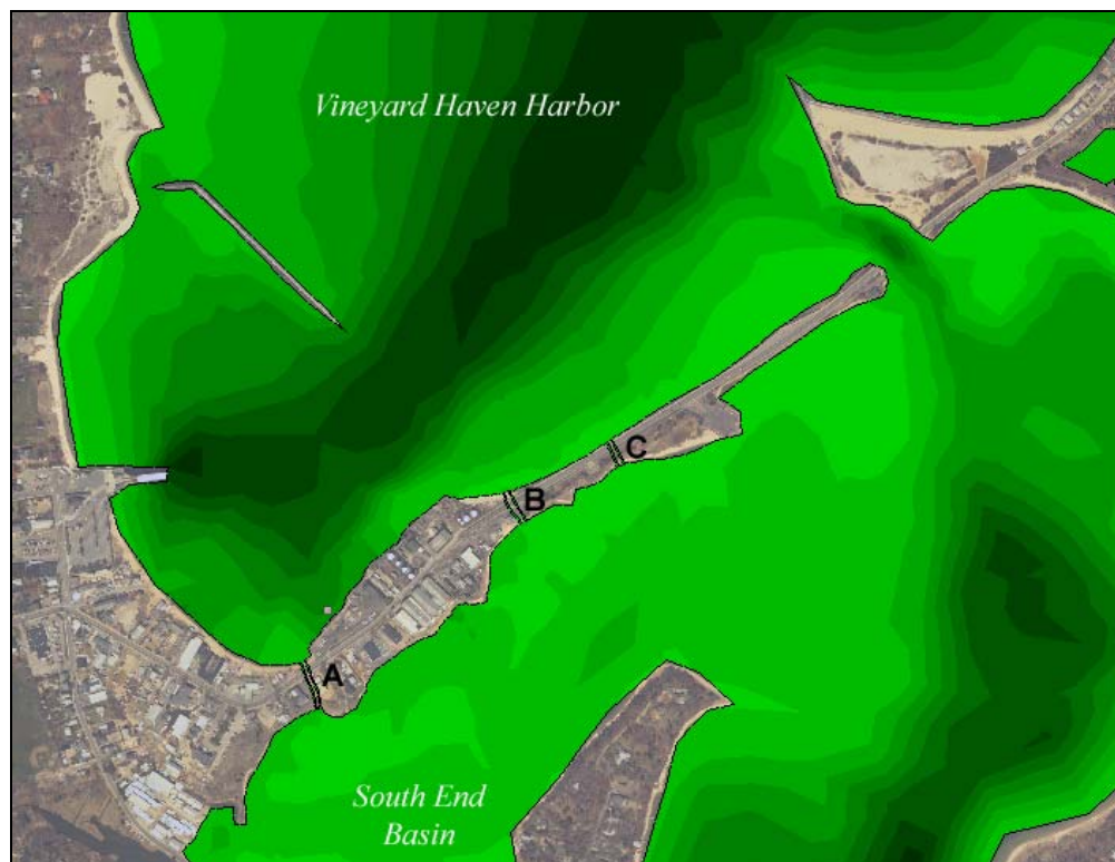
Figure IX-1. Location of six culverts (two each at A, B and C) placed in the hydrodynamic model of Lagoon Pond to investigate possible water quality improvements.
