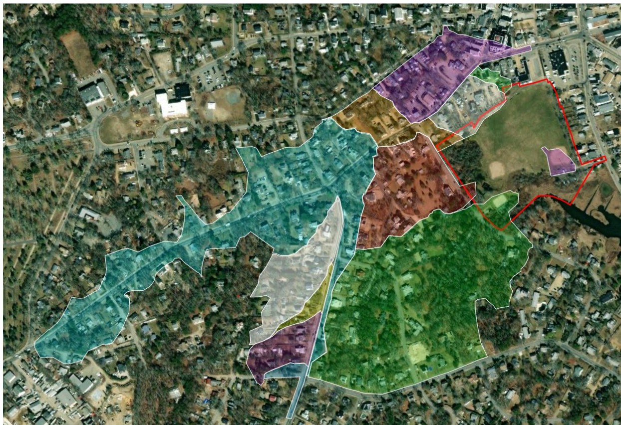
Figure 3 Drainage Areas for Proposed SCMs
