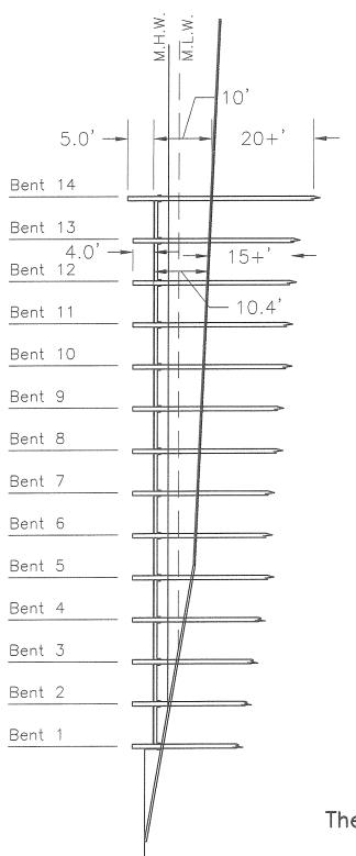
Piles at Bent 14 shall Piles at Bents 1—13 shall be cut off 4 ft. be cut off 5 ft. above the deck elevation.
